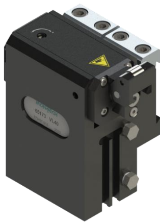
Separator VL40 – with pawl with spring reset for stopping and separating accumulating workpiece carriers e.g. as a pre-stopper upstream from a positioning unit
