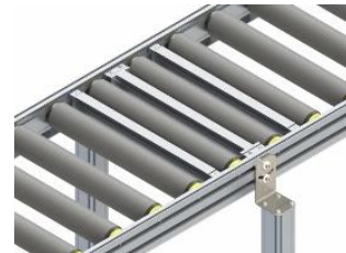
connection for roller conveyors longer than 3 m
